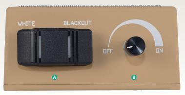
**INSPECT** the control panel carefully. Make sure the lighting control dial turns smoothly and clicks off and on. Then check the LED toggle, listening for a hard click at each setting.
